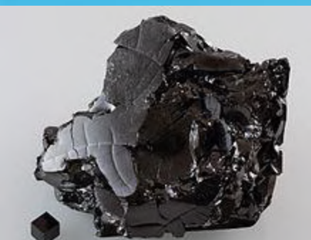
large sample of glassy carbon, with 1 cm 3 graphite cube for comparison
